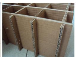
\*Difference between internal dividers with horizontal fluting (correct) and vertical fluting (wrong)
