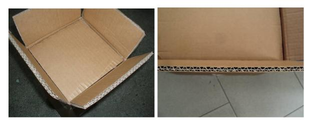
Examples of internal dividers and air cells. Carton double wall 5 ply with <u>horizontal flute direction\*</u>. 6,48 mm thickness:
